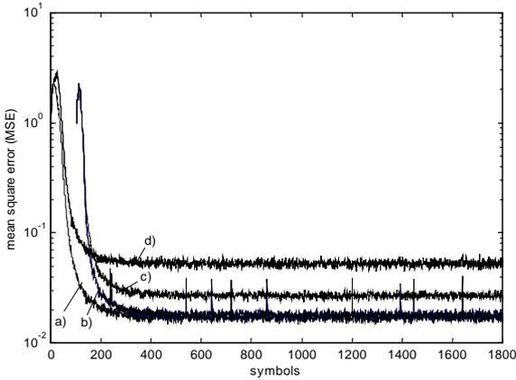
Fig. 4: convergence rate for 2 user SDMA/TDMA system: a) noSIC u1, b) idealSIC u2, c) corSIC u2 and d) noSIC u2
