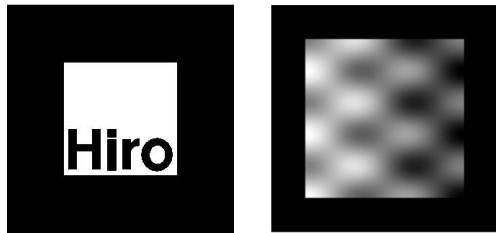
Figure 1: A sample template from the ARToolKit distribution (left) and from the maximum distance set (right).
