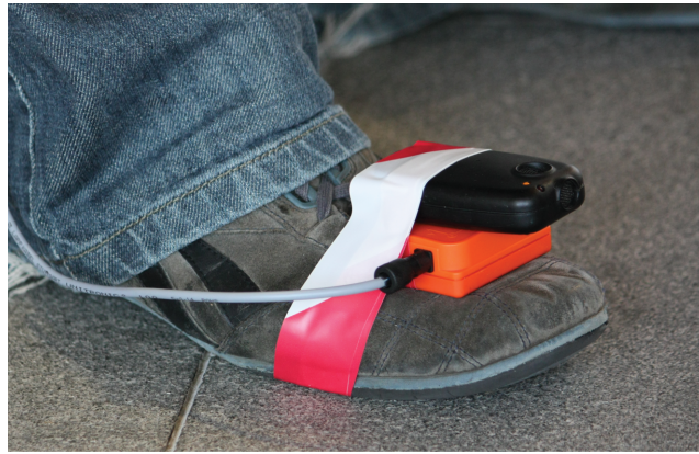
Figure 4.8: An Active Bat mounted above an Xsens IMU on the user's foot.
