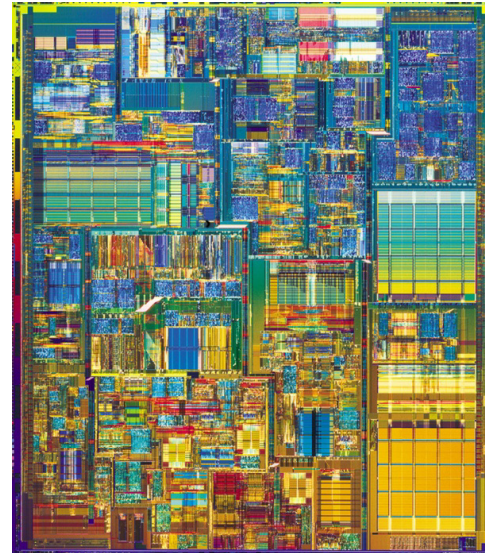
Intel Pentium-4 (2000) 42,000,000 transistors 0.18 \mu m process
