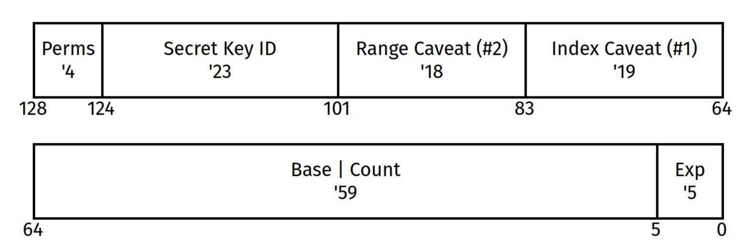
The 128-bit IOCap text format. The first 64-bits encode an initial resource, with up to 1KiB granularity, which can be refined to 1B granularity using the caveats. This must be accompanied with a 128-bit signature (not shown), which is the end result of an hash chain starting at the **secret key** ID-d by the capability, similar to Macaroons (shown below).
