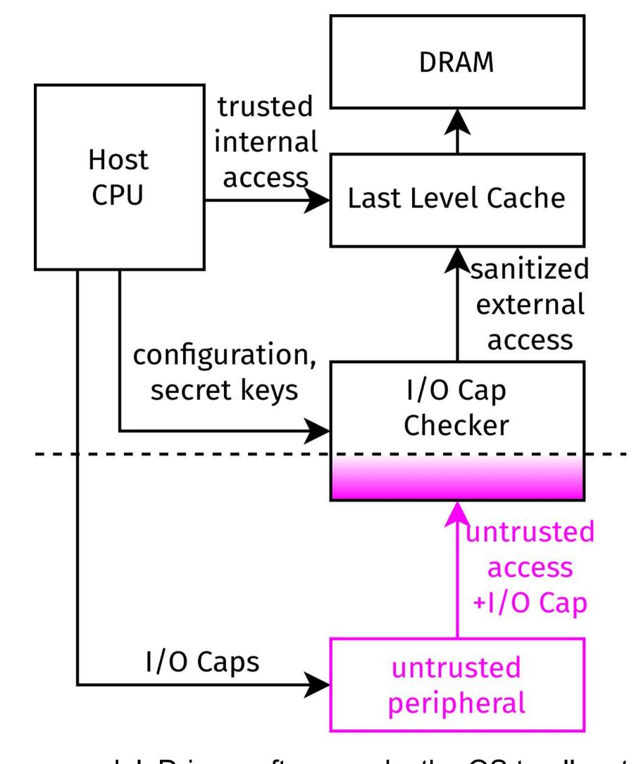
The IOCap usage model. Driver software asks the OS to allocate secret keys and generate IOCaps. Peripherals are given IOCaps to grant access to different ranges of RAM, and must present them with each attempted DMA access. The combined signature & plaintext prevent tampering.
