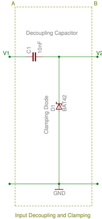
Figure 1: Input Decoupling and Clamping Stage
