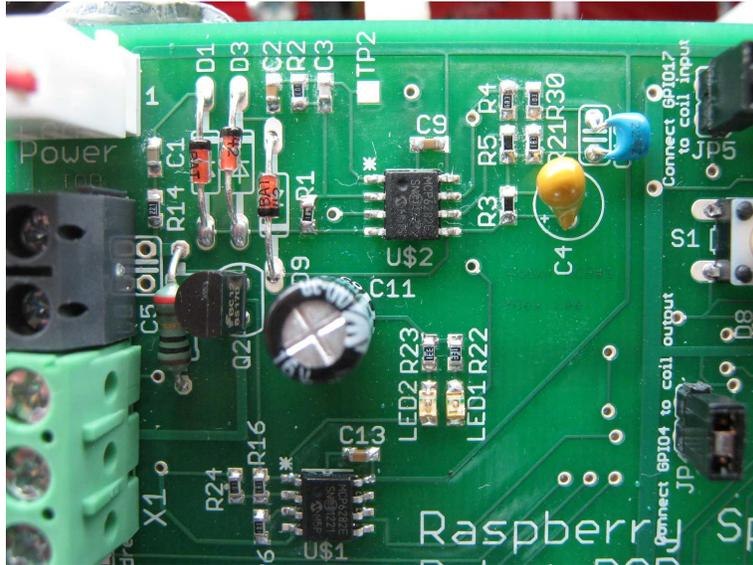
Figure 10: Receiving and Transmitting Circuits on PCB
