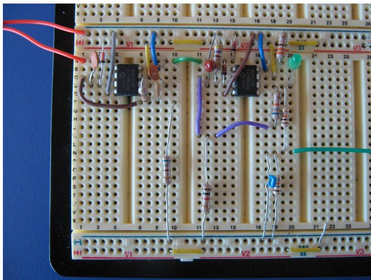
Figure 11: Receiving Circuit on Solderless Breadboard
