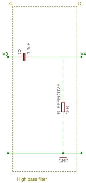
Figure 3: High Pass Filter
