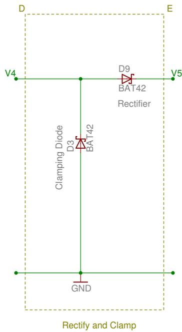
Figure 4: Rectifier and Clamping
