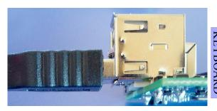
To connect your (USB) keyboard to the Pi, put the end of the cable into the space as shown opposite.
