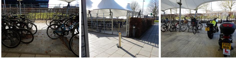
Figure 1: (a) Substandard aisles (b) Obstructed entry (c) Motorcycles
