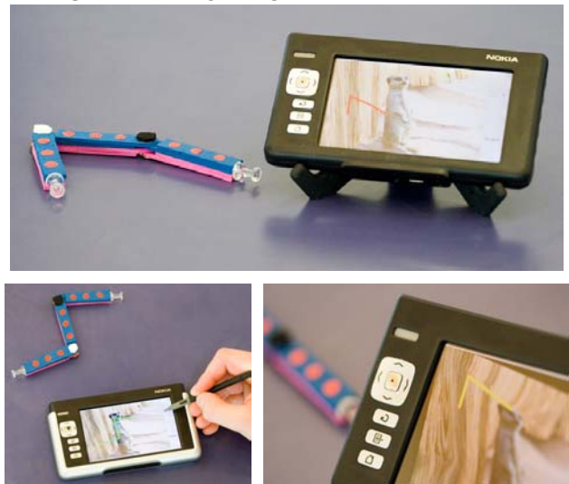
Figure 4 - a) articulated tangible device; b) selection of image warp mode; c) warped image
