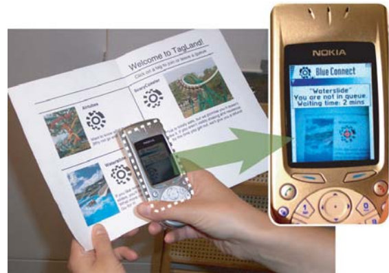
Figure 2 – Bimanual interaction between camera-phone and visual tags on printed leaflet (result of previous project with Intel Research)
