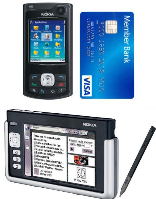
Figure 1: a) N80 smartphone and b) N770 internet tablet, shown approximately to scale, with standard credit card for comparison.
