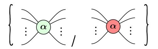
You can draw any quantum circuit using just these two types of spiders.
