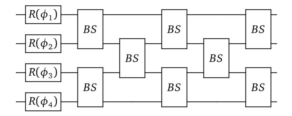
An example 4-mode interferometer
