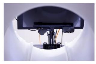
Figure 1. EyeLink 1000 Plus long-range eye tracker, mounted under the MRI viewing monitor.
