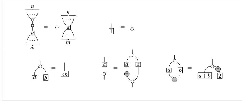
Here the two rules on the left are generalisations of rules of the parameter-free setting, while the other three rules relate operations of the ring to certain diagrams. We show that our proof of completeness of the parameter-free ZH-calculus extends to this setting, making  $ZH_R$  complete over the set of  $2^n \times 2^m$  matrices with entries in  $R$ .
