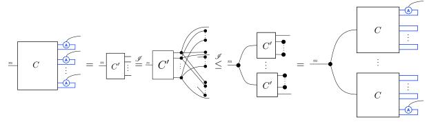
The diagram above illustrates this for ammeters, but it applies to any mixture of meters, remembering that a discarded voltmeter is an open circuit. If moreover each individual measurement is a function of the inputs (i.e. single-valued and total), then the inclusion is an equality.
