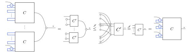
The diagram illustrates this with voltage sources, but it applies to any mixture of sources, given that a turned off current source is an open circuit. If moreover the outputs are a function (i.e. single-valued and total) of each source when activated individually, then the inclusion is an equality.
