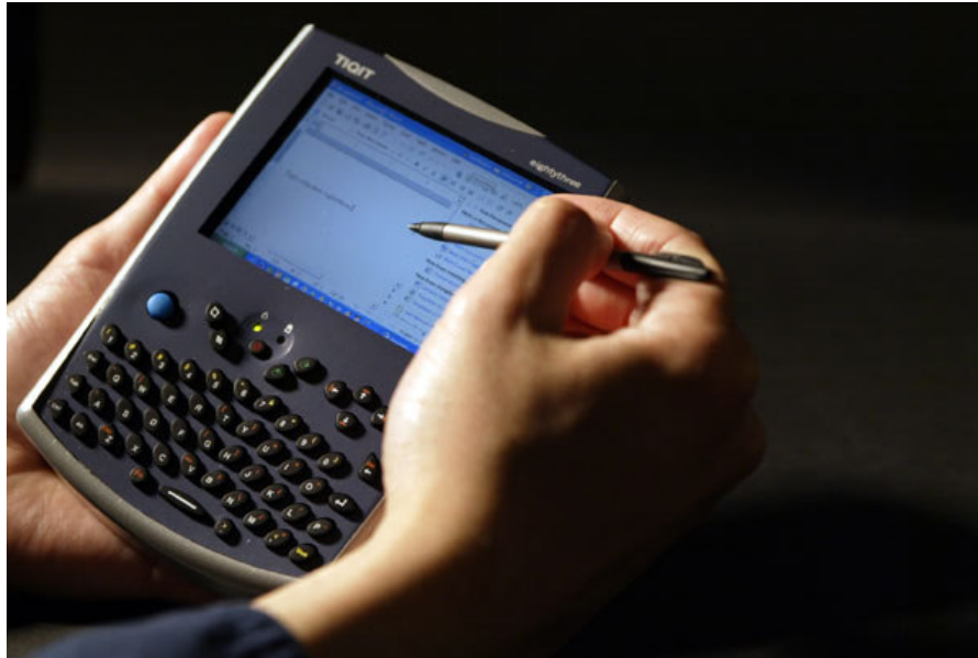
Figure 3: The Tiqit Eighty Three Computer. This device provides a keyboard, a joystick and a stylus for user interaction.
