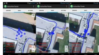
The app in action – the white line is without opportunistic sensing and SLAM, the blue line is the full SLAM solution
