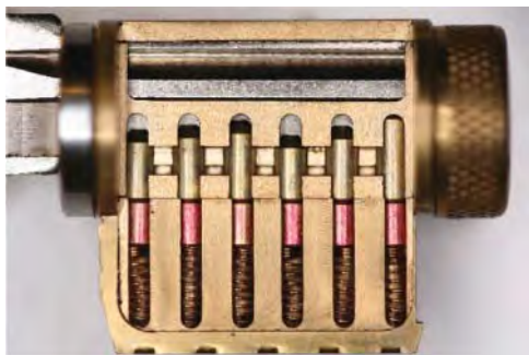
Figure 13.1: A cutaway pin-tumbler lock (courtesy of Marc Weber Tobias)
