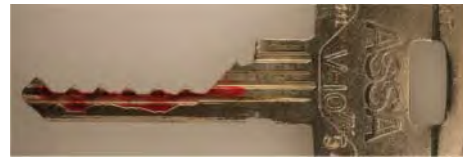
Figure 13.3: Sidebar bump key
