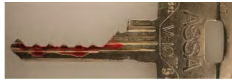
Figure 13.3: Sidebar bump key
