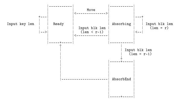
The function MITB is similar MITB\_FUN except that it decodes the inputs into abstract commands Skip, Move and Input  $bk \ len$ .
