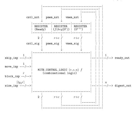
This diagram is expressed in logic in a standard way using relations.<sup>7</sup> Melham's book is a comprehensive reference [10]. The definition of MITB below uses the relation REGISTER to model registers as a unit delay:
