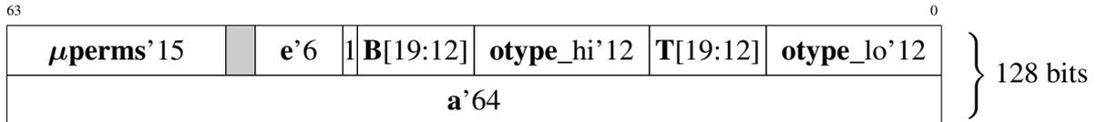
Figure E.6: Sealed CHERI-128 memory representation of a capability
