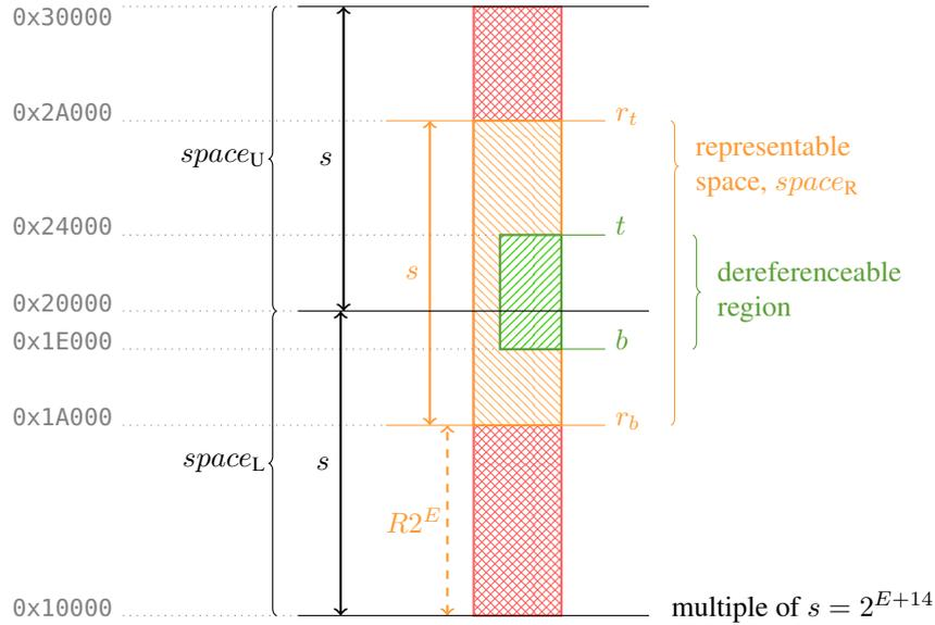
Figure 3.3: Graphical representation of memory regions encoded by CHERI Concentrate. The example addresses on the left are for a  $0x6000$ -byte object located at  $0x1E000$ ; the representable region extends  $0x4000$  below the object’s base and  $0x8000$  above the object’s limit.
