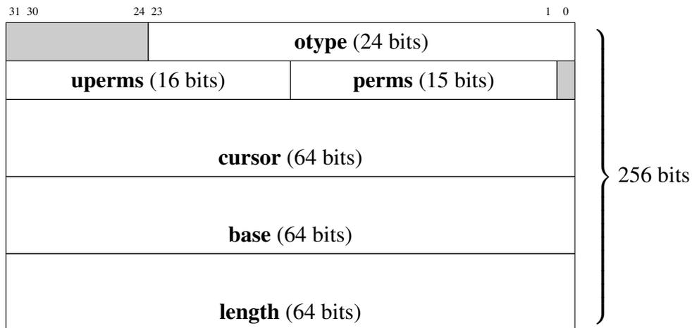
Figure 3.1: 256-bit memory representation of a capability
