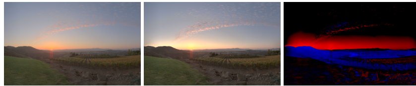
Figure 25: Image tone mapped using logarithmic mapping [37] (left), its version with restored global contrast (center), and the corresponding map of Cornsweet profiles (right). The blue profiles darken the image and the red lighten, their intensity corresponds to the profile magnitude. Note that the contrast restoration preserves the particular style of the tone mapping algorithm. (Images courtesy of Grzegorz Krawczyk. Reproduced with permission from [72] © The Eurographics Association 2007.)
