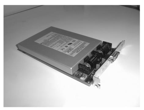
Figure 16.1: The IBM 4758 cryptoprocessor (courtesy of Steve Weingart)
