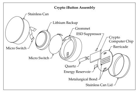
Figure 16.3: iButton internals (courtesy of Dallas Semiconductor Inc.)
