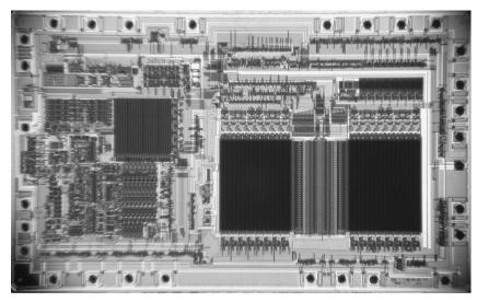
Figure 16.7: MC68HC705P6A microcontroller (courtesy of Sergei Skorobogatov)
