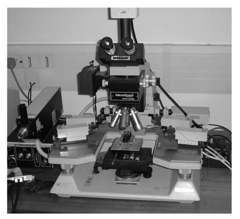
Figure 16.4: Low-cost probing station
