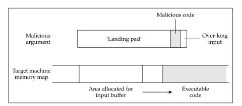
Figure 4.6: Stack smashing attack
