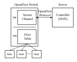
Figure 2.1: OpenFlow switch and controller setup [13]
