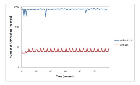
Figure 4.4: Graph depicting the number of ARP packets that can be exchanged between two hosts per second.
