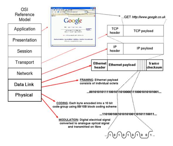
Figure A.1: OSI model of network protocol layers. Adapted from [25, Figure 1.1]
