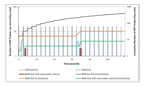
Figure 4.2: Graph showing the rate and the cumulative total of ARP messages exchanged by a host using different ARP mechanisms
