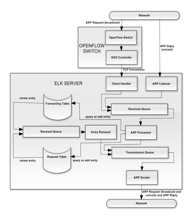
Figure 3.2: Flow chart diagram showing the processing path taken by the incoming packets.
