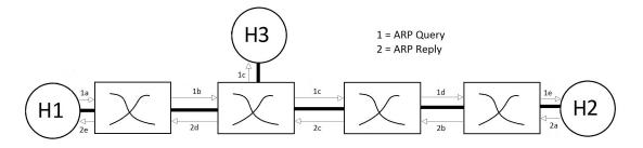
Figure D.1: ARP in simple line topology - 4 switches, 3 hosts, 6 ARP queries and 5 ARP replies
