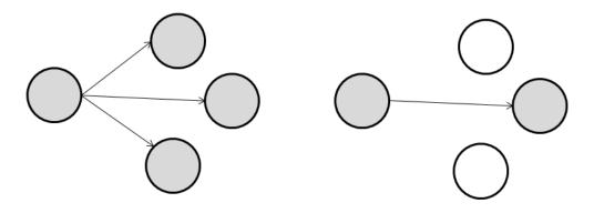
Figure 1.1: Broadcast (left) and Unicast (right)
