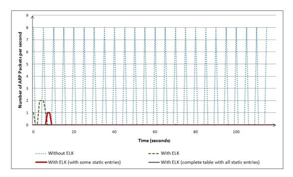
Figure 4.3: Graph showing the rate of broadcast ARP messages received by a host using different ARP mechanisms
