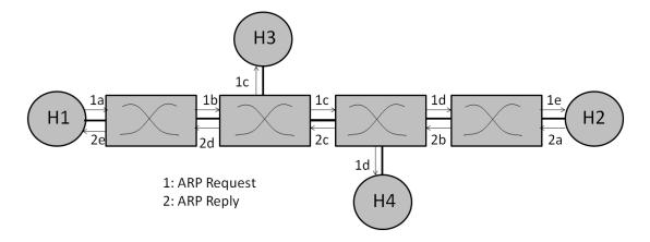
Figure 1.4: Network View of ARP Transaction
