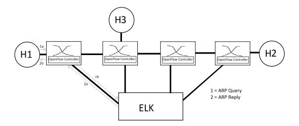
Figure D.2: ARP with ELK in line topology - 4 switches, 3 hosts, 2 ARP queries and 2 ARP replies
