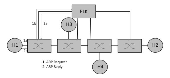
Figure 1.5: Conceptual Network View of ARP Transaction with ELK
