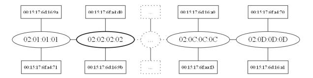
Figure 4.1: Network topology of first MOOSE forwarding table size experiment, 12 switches in total. Ellipses indicate switches, boxes indicate hosts
