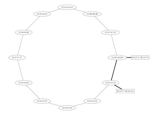
Figure 4.8: MOOSE network topology of optimal routes experiment — Bold links show route taken
