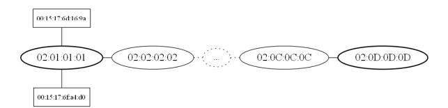
Figure 4.3: Network topology of second MOOSE forwarding table size experiment, 12 switches in total. Ellipses indicate switches, boxes indicate hosts
