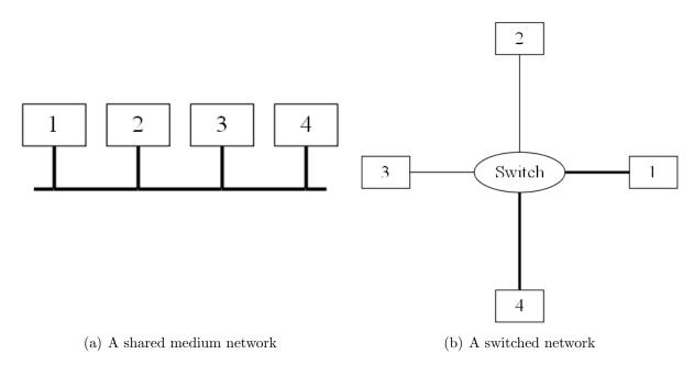
Figure 1.2: Comparison of shared-medium and star network topologies Bold links are those used (thus not free for other use) when 1 and 4 communicate
