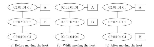
Figure 4.10: Topology of network for host mobility experiment
