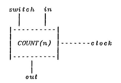
When the counter is clocked, the new value of the state variable n becomes n+1 (i.e. the old value plus one) if *false* is being input on line *switch*, otherwise it becomes the value input on line *in*. We can express this by:
