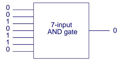
Feed sets of arguments in as inputs, and check whether the output is as expected.
