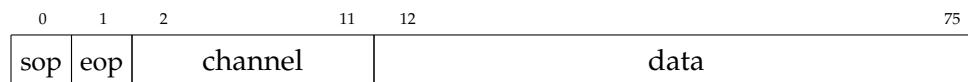
Figure 7.12: Layout of a link layer flit. sop and eop stand for “start of packet” and “end of packet” respectively
