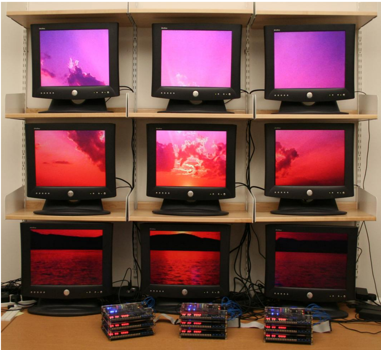
Figure 3.4: A display wall based on the computing surface architecture
