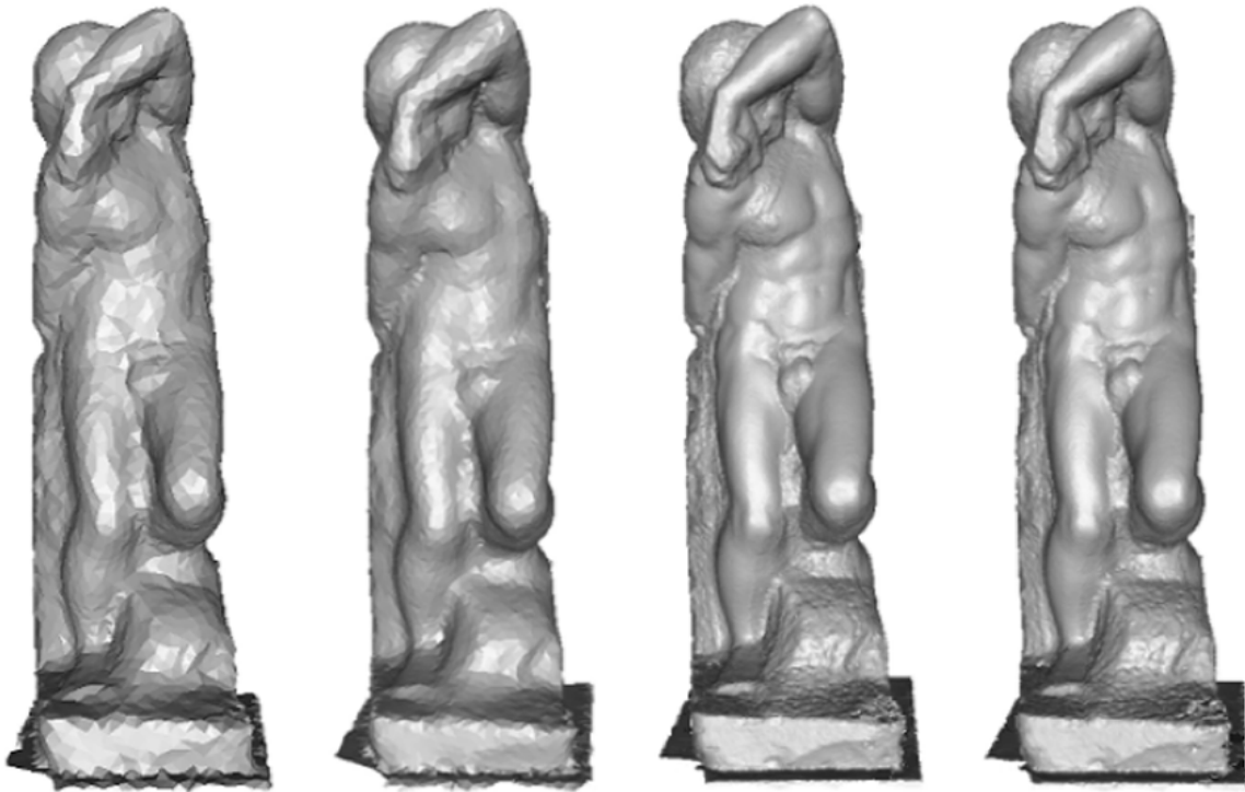
Figure 4.10: Level-of-details of the Michelangelo Youthful data set (1728305 points) produced from point sets generated by progressive uniform resampling of the original point cloud to 0.25%, 0.5%, 1.0% and 5.0% of its size ( from left to right ).
