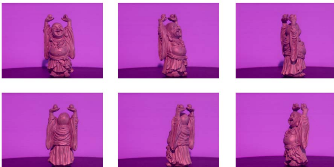
Figure 4.5: Optical acquisition of a Buddha sculpture using laser range scanning. The object was rotated by 60 degrees after each range shot taken with a Minolta VIVID-900 laser scanner. The scanner’s precision of 0.02mm resulted in a representation of the sculpture’s surface consisting of 152154 points. This representation was affected by artefacts due to shortcomings inherent to optical acquisition and suboptimal acquisition conditions.
