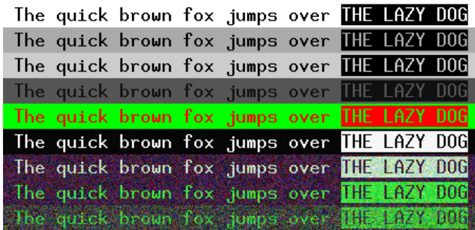
Figure 4.9: Example test image for text contrast in compromising emanations from DVI cables.
