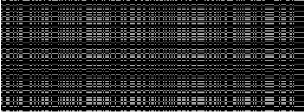
Figure 4.7: The text “Tempest in a Teapot” encoded in ASCII (padded with start- and end-of-text control characters) DSSS-modulated.
