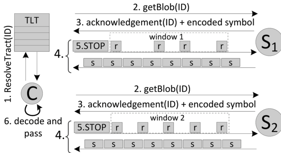
Figure 4.3: Trevis reads data from multiple sources using a pull-based transport API
