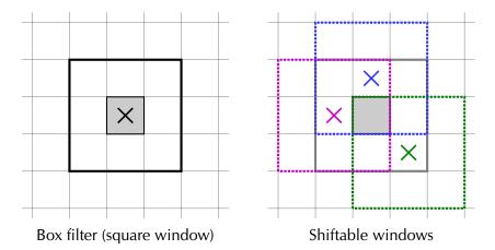
**Figure 2.12:** Comparison of the box filter and shiftable windows cost aggregation techniques. **Left:** The box filter accumulates costs inside the 3×3 window centred on the shaded pixel. **Right:** The box filter is shifted across pixels in the solid grey window, and the minimum cost is taken. Three dotted windows are shown centred on different pixels (indicated by crosses).
