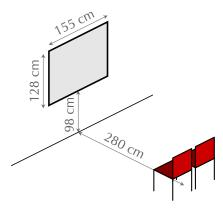
**Figure 6.4:** Experimental setup for the perceptual study.
