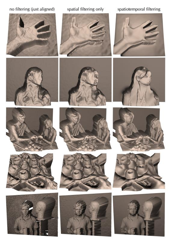
**Figure 4.8:** Mesh renderings of distance maps without filtering, with spatial and spatiotemporal filtering. It is essential to refer to the supplementary video to see the full improvement in quality. The last row shows data captured using a Microsoft Kinect, with holes and the characteristic depth quantisation steps. This chapter's filtering approach results in a clear improvement.
