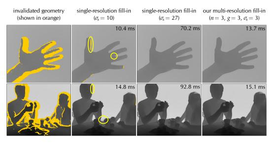
**Figure 4.4:** The multi-resolution geometry fill-in technique is  $5-6 \times$  faster than the single-resolution fill-in with the large kernel size ( $\sigma_s = 27$ ) necessary to fill holes, with comparable quality. A smaller kernel ( $\sigma_s = 10$ ) has a similar run time, but shows errors (highlighted in yellow).
