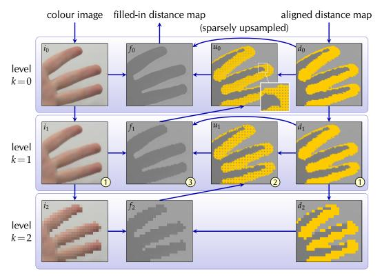
**Figure 4.5:** Illustration of the multi-resolution geometry fill-in technique using the 'hand' sequence (with parameters  $n = g = \sigma_s = 3$ ). Please refer to Section 4.2 for a step-by-step explanation.
