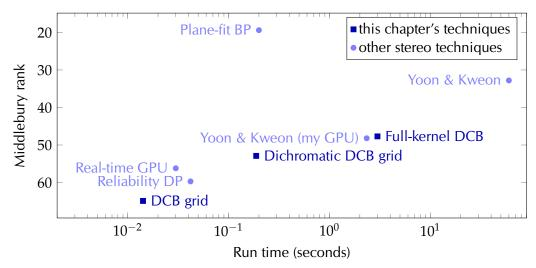
**Figure 3.5:** Scatter plot visualisation of run time (Table 3.2) versus Middlebury rank (Table 3.3) for the techniques presented in this chapter and other stereo matching techniques. Most techniques lie close to a straight line which trades off run time and Middlebury rank.
