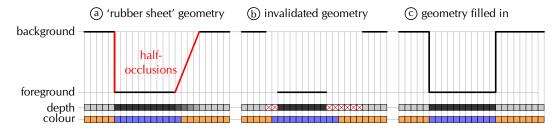
**Figure 4.3:** Illustration of the geometry fill-in procedure on a slice of scene geometry as seen from above: (a) 'rubber sheet' with half-occlusions; (b) after geometry invalidation; (c) with geometry fill-in.
