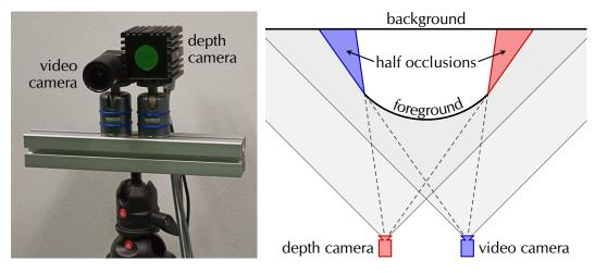
Figure 4.2: Left: The prototype camera setup with video and depth cameras mounted on a tripod. **Right:** Schematic of the camera setup, with highlighted half-occlusion areas.
