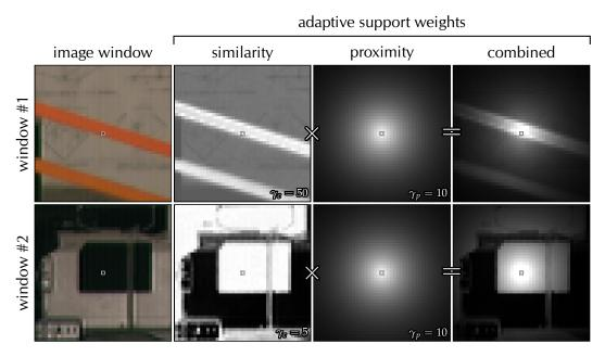
**Figure 3.1:** Computation of adaptive support windows (Yoon and Kweon, 2006) for two pixels from the *Tsukuba* stereo image. The pixel position is marked by a rectangle in the centre of the windows. Lighter shades indicate higher weights.
