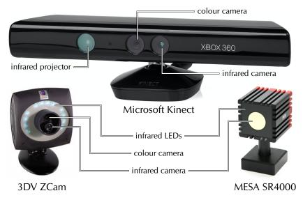
Figure 2.11: Three commercial depth sensors and their components (not to scale).
