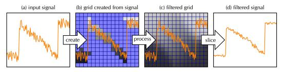
**Figure 3.2:** Illustration of 1D bilateral filtering using the bilateral grid: the signal (a) is embedded in the grid (b), which is processed (c) and sliced to obtain the filtered signal (d). Please see Section 3.2.1 for details. Adapted from Chen et al. (2007).
