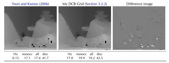
**Figure 3.7:** Comparison of cost aggregation techniques in Yang et al.'s spatial-depth super-resolution on 8× sub-sampled *Teddy*. My DCB grid is more than 100× faster, at only a small loss of quality.
