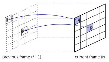
Figure 4.6: Illustration of the motion-compensated filter kernel: arrows indicate optical flow from the kernel centre **p** and a kernel pixel **q** in the current frame (t, right) to the previous frame (t-1, left).
