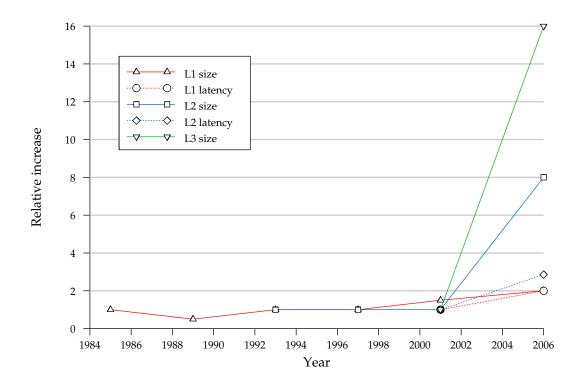
Figure 2.3: Relative increases of cache size and latency, 1984—2006
