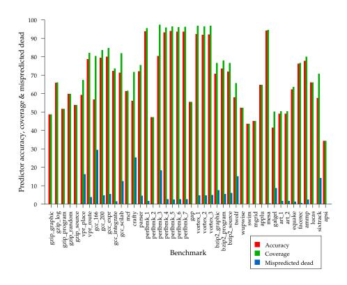
Figure 5.33: AccessInterval\_2SAddr predictor performance
