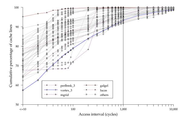
Figure 3.14: Cumulative distributions of access intervals for the IL1 cache
