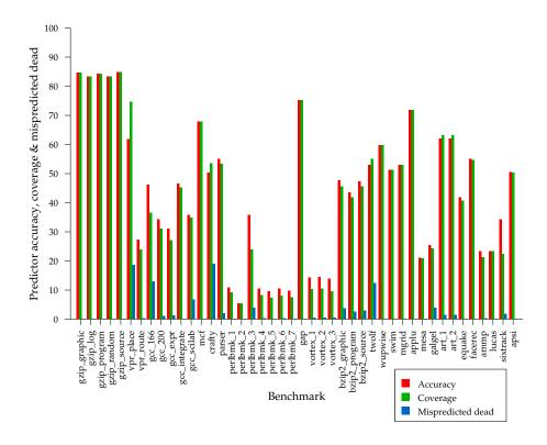
Figure 5.25: LastTouch\_1PC2Addr predictor performance
