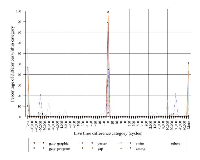
Figure 4.4: Distributions of live time differences for the L2 cache
