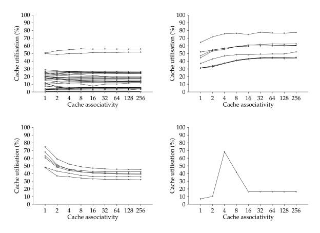
Figure 3.25: Cache utilisation *vs* cache associativity for the DL1 cache. Similar trends are clustered into four different groups (A, B, C, D) from top-left to bottom-right.
