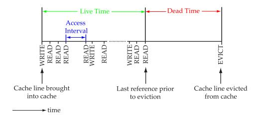
Figure 3.6: Cache line lifetime metric definitions
