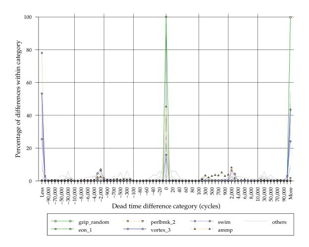
Figure 4.7: Distributions of dead time differences for the L2 cache
