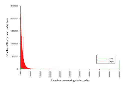
Figure 5.10: Distribution of live and dead cache lines in the victim cache clustered by live time for <code>gzip\_graphic</code>
