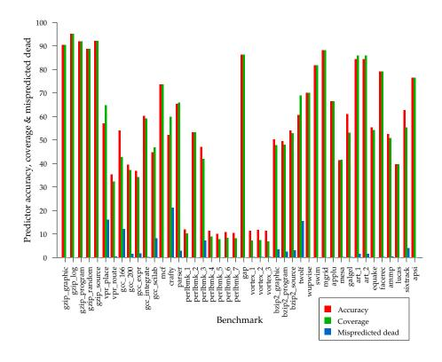
Figure 5.23: LastTouch\_2SAddr predictor performance
