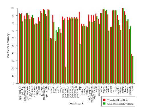
Figure 5.11: Accuracy of the ThresholdLiveTime and DualThresholdLiveTime predictors
