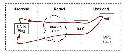
Figure 5.4: Architecture of our evaluation setup; the red line shows the data path of a single ICMP echo packet through the kernel into the user-level stack being evaluated.
