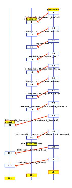
Figure 7.9: The SPIN guided backtrace for the shortest possible violation of an LTL specification (see text for details)
