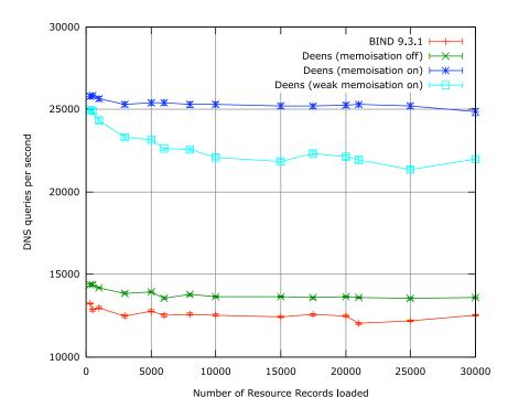
Figure 7.13: Query performance of BIND 9.3.1 versus deens running in three modes: (*i*) memoisation off; (*ii*) memoisation using a space-leaking hash-table; and (*iii*) memoisation using a safe weak hash-table cache.
