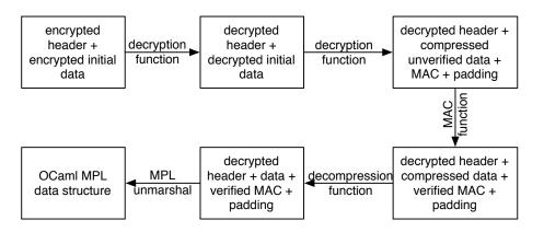
Figure 7.6: SSH unmarshal path for a single packet which shows the sequence of decryption, decompression, MAC verification and finally classification of the contents with MPL
