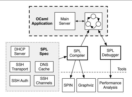
Figure 6.1: The SPL tool-chain architecture
