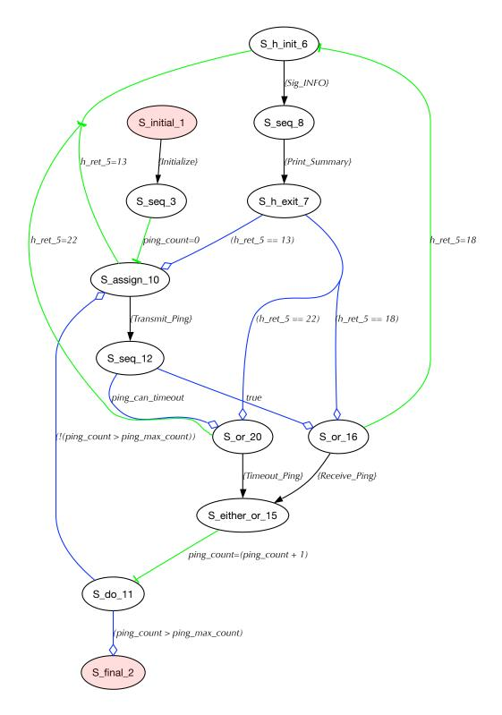
Figure 6.2: Graph output of the example ping state machine. Red nodes indicate the start and final states, black edges are statecalls, blue edges are conditional, and green edges are state variable assignments
