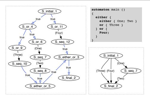
Figure 6.8: Conditional elimination on a CFA (left) before, and (right) after
