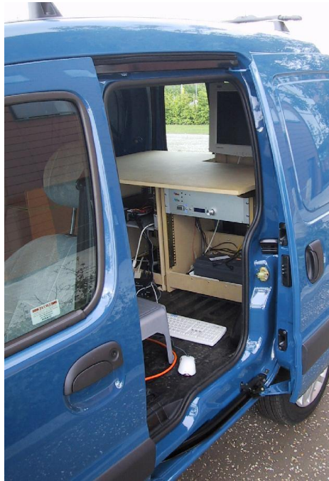
Figure 3.1: View through the side door of the vehicle, showing the placement of the equipment rack.
