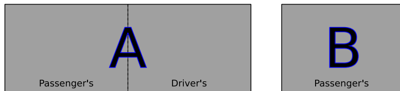
Figure 3.7: Two VNC desktops, with A twice the width of B. Desktop A is divided into two halves, one for passenger and driver each. Desktop B is the passenger's independent desktop.
