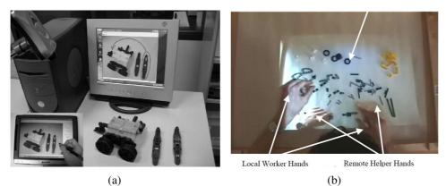
Figure 2.6: Examples of remote gesture technologies: (a) using sketching (from Fussell et al., 2004); and (b) using an unmediated video representation of the hands (from Kirk, 2007).
