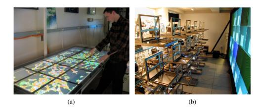
Figure 3.5: Increasing display resolution by tiling: (a) LCD panel displays (from Krumbholz et al., 2005); and (b) projectors (from http://www.cs.princeton.edu/omnimedia).
