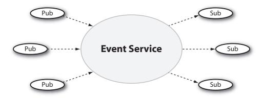
**Figure 1.1**: A publish/subscribe systems consists of a number of publishers and subscribers and an event service decoupling the two from each other.
