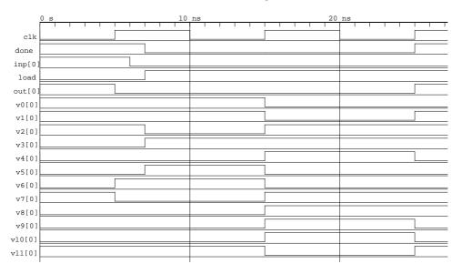
Figure 4.2: Well-behaved simulation with combinational loop.
