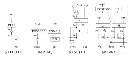
Figure 2.10: Implementation of composite devices.
