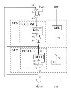
Figure 4.1: Combinational loop in (SEQ (ATM  $(\lambda x. x)$ ) (ATM  $(\lambda x. \neg x)$ )).
