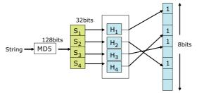
Figure 6.15: Bloom Filters for String constraint
