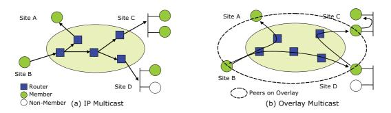
Figure 2.5: IP Multicast and Overlay Multicast
