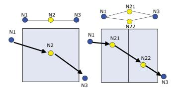
Figure 5.5: Splitting a space for load balancing in Meghdoot
