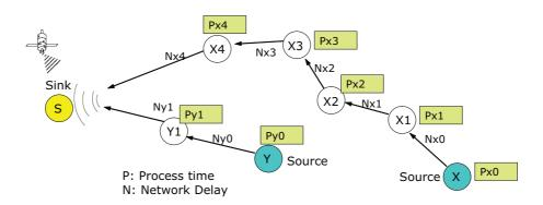
Figure 7.16: Lightweight Local Clock Propagation
