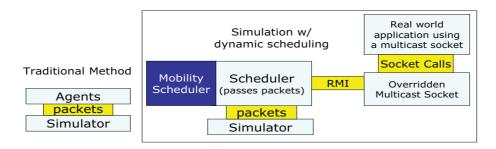
Figure 6.25: Components Structure of Simulator
