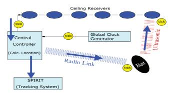
Figure 7.39: Time Synchronisation Mechanism in Active BAT and SPIRIT
