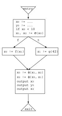
Figure 3.4: When to place  $\sigma$ -functions (2)
