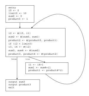
Figure 5.9: Example SSI program to be sliced
