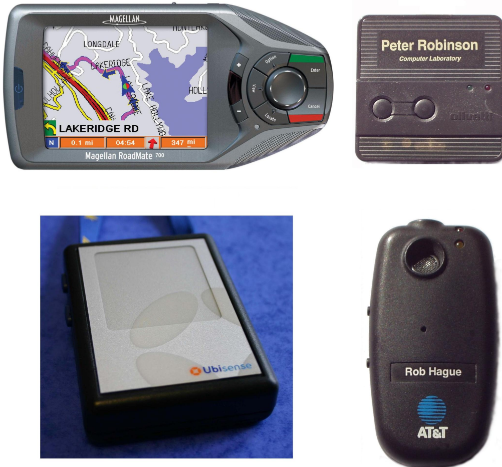
Figure 2.1: Positioning technologies. Clockwise from top left: a GPS receiver, an Active Badge, an Active Bat, and an Ultrawideband tag (not to scale)
