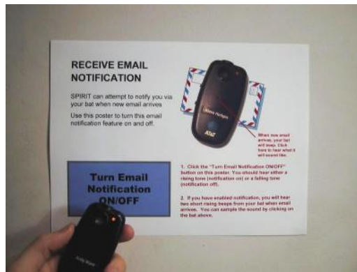
Figure 2.3: Posters such as this one are located on walls. Bringing the Bat close to the corresponding “button” (thick-bordered rectangle) and “clicking” will send a command to the environment.
