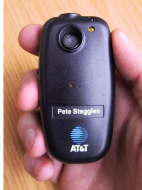
Figure 6.1: The Bat is a small device that is about 85 mm long. Two buttons are located on the left side.
