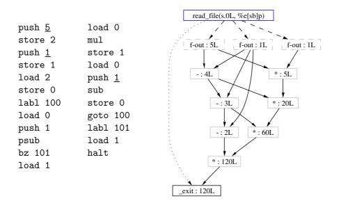
Figure 5.5: DDFG for iterative fac(5) on an interpreted stack machine
