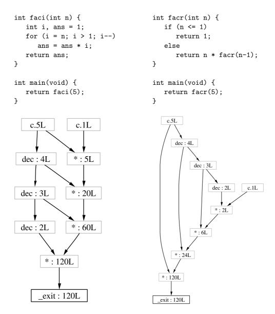
Figure 5.1: DDFGs for iterative and recursive fac(5) in C  $\,$
