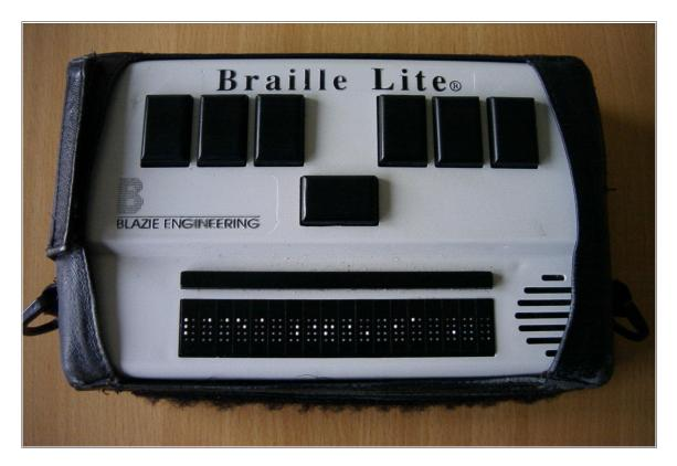
Figure 5.30: Braille-based note-taking device (photo: Hans Schou)
