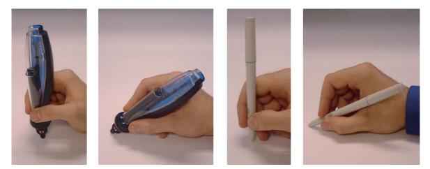
**Figure 7.7:** Holding the pens obliquely can cause problems. The Mimio pen reports variations in position of up to 15mm in each direction if it is held at very acute angles (left two images). The digitizer pen's nib button can be difficult to engage when it is held obliquely (right two images).
