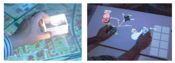
**Figure 2.19:** The metaDESK [UI97] and Sensetable [PIHP01] projects from the Tangible Media Group at MIT. They are examples of tangible user interfaces where physical objects allow many parameters of a system to be controlled with minimal effort spent switching between parameters.
