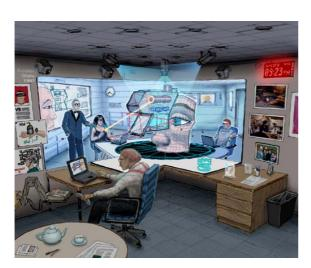
**Figure 2.12:** A sketch of the Office of the Future [RWC<sup>+</sup>98]. The researchers envisage a multitude of inexpensive cameras and projectors embedded in the office. The cameras infer the geometry and reflective properties of the visible surfaces and the projectors create 3D imagery on them for a user whose eye positions are tracked in 3D.
