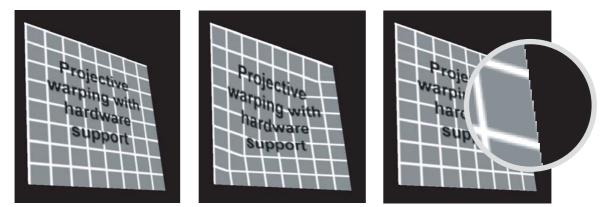
**Figure 4.8:** Errors that can occur when using video hardware for projective warping: (left) the correctly warped image; (centre) the homogeneous W co-ordinates for the vertices have not been used, resulting in inconsistent warps for the two triangles that comprise the image; (right) the texture co-ordinates have been set too high on the right and bottom edges, resulting in the texture beginning to wrap and stray pixels appearing along the those edges.
