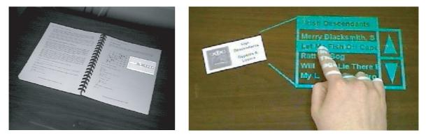
**Figure 2.16:** The LivePaper system [RR01]. A book (left) is augmented with projected graphics to add *literal functionality* that augments the pictures on the page. A card (right) invokes an associated menu to play songs, which demonstrates *magical functionality* that is not related to the normal physical properties of the card.
