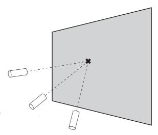
**Figure 5.9:** To calibrate the wall display a target is displayed on the surface and the user must aim at it from several locations so that an estimate of its 3D location can be obtained.
