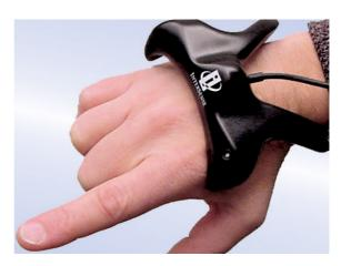
**Figure 8.1:** The Intersense MiniTrax ultrasonic hand tracker [MT]. A device like this would avoid the problems that a magnetic tracker has with metal objects, and would leave the hand free to hold a pen.
