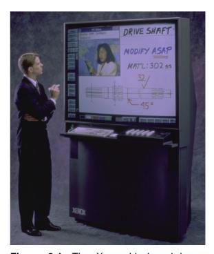
**Figure 2.4:** The Xerox Liveboard is an example of a large display device. The original was a  $4 \times 3$  foot,  $1120 \times 780$  pixel, rear-projected display driven by the X Window System and controlled by a laser pentracked by a camera behind the screen [EBG<sup>+</sup>92].
