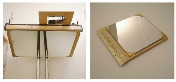
**Figure 3.7:** In the first version of the Escritoire hardware the projector for the fovea (left) was placed on top of the shelf above the desk that holds the large mirror, and had a smaller mirror (right) that reflected it's image down onto the desk surface.
