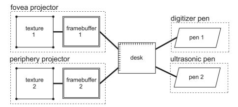
**Figure 4.4:** Co-ordinate spaces for multiple input and output devices. These are the coordinate spaces used for the Escritoire's desk display, which has projectors for the fovea and periphery, and a pen for each of the user's hands. The single desk space where graphical objects are arranged links the system together.
