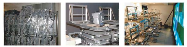
**Figure 2.11:** The Princeton display wall: (left) the cluster of PCs that drive the projectors, linked by a fast network; (centre) a projector on its mounting that has six degrees of freedom and a shadow mask to restrict the projected image to an adjustable rectangular area; (right) the array of 24 projectors.
