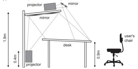
**Figure 3.6:** The two-projector arrangement of the foveal display. A shelf above the desk holds one projector that reflects its image in a small mirror to make the fovea. Another projector that is mounted behind the desk reflects its image in a large mirror on the bottom of the shelf to make the periphery. The height and angle of the shelf are adjustable. The measurements are approximate.
