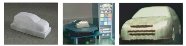
**Figure 2.13:** Projections can be made onto complex objects rather than flat surfaces. In augmented prototyping [VdSPvG03] a model of a car is augmented with projected graphics. The user chooses attributes, such as the paint colour, from a projected menu, and views the results on the model.
