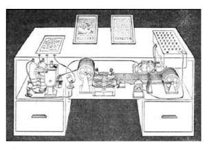
**Figure 2.17:** Vannevar Bush imagined a device called the Memex [Bus45] in the form of a desk that would instantly bring files and material on any subject to the operator's fingertips. Slanting translucent viewing screens magnify supermicrofilm filed by code numbers. On the left is a mechanism that automatically photographs longhand notes, pictures, and letters, then files them in the desk for future reference.
