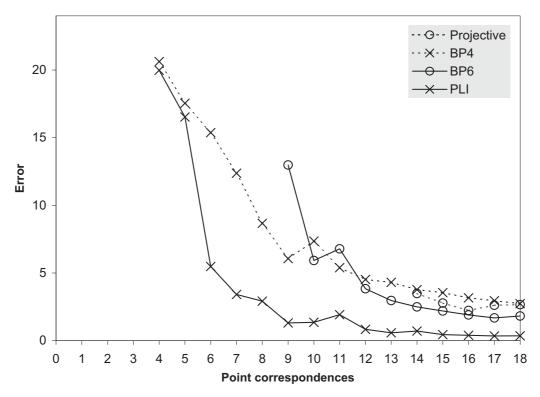
**Figure 5.8:** Four mappings applied to ultrasonic pen data. Average error in pixels is plotted against number of point correspondences used to initialize the mapping. The error from PLI reduces rapidly as correspondences are added, and it achieves the lowest level.
