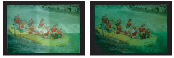
**Figure 2.14:** Photometric calibration of a multi-projector display [MS03]. Without calibration (left) the  $2 \times 2$  projector array is much brighter in the overlap regions. The images from the projectors are selectively attenuated (right) to achieve uniform brightness across the whole display.
