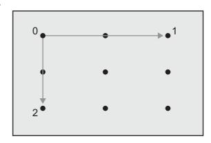
**Figure 5.10:** Creating a co-ordinate frame on the 3D plane: the 3D locations of targets 0 and 1 from the framebuffer are used to create a horizontal axis on the plane, and those of targets 0 and 2 to create a vertical axis.
