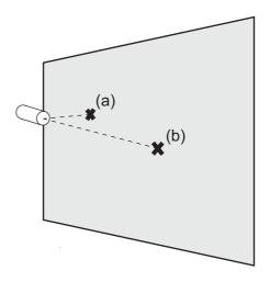
**Figure 3.4:** Generating a 2D event from the wand's location and orientation: (a) we can project the location orthogonally onto the plane, or (b) we can intersect a line through the wand with the plane.
