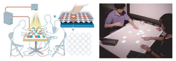
**Figure 2.21:** Prototype electrical touch sensing technologies: (left) DiamondTouch [LD02]; and (right) SmartSkin [Rek02]. Both devices use a grid of wires embedded in the surface to track multiple hands.
