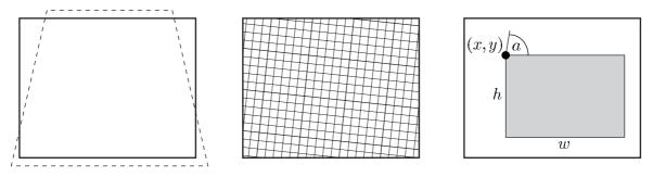
**Figure 4.7:** Positioning the display rectangle on the surface: (left) the projector's field of view will not coincide with the surface; (centre) in general the pen co-ordinate system will not be aligned to the surface; (right) the user picks the location (x, y), size (h, w), and angle *a* of the display to make best use of the surface.
