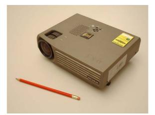
**Figure 3.1:** Projectors are getting smaller and cheaper. This is a Proxima DX3: dimensions  $245 \times 195 \times 68$  mm, weight 2.3 kg, resolution XGA (1024 × 768), brightness 1100 lumens, cost under 2000 euros.
