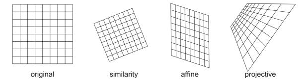
**Figure 5.1:** Three global mapping functions that could be used to calibrate a pen input device. A similarity transformation scales, rotates and translates the grid, an affine transformation also performs non-uniform scaling and shears, and a projective transformation adds perspective effects.
