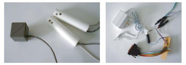
**Figure 3.3:** Wands containing magnetic trackers: (left) the magnetic emitter, and the plastic tubes of the wands that contain the magnetic receivers and buttons; (right) the wiring used to sense the button presses via the computer's parallel port.
