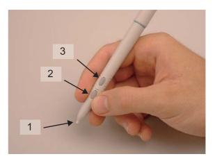
**Figure 7.6:** The digitizer pen for the dominant hand has three buttons: one in the nib, and two on the shaft. How combinations of buttons are interpreted by the software must be designed carefully.
