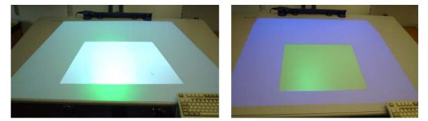
**Figure 4.6:** Before calibration (left) the output of the projectors is distorted due to oblique projection so the images will not appear rectangular. After calibration (right) the projected images are warped to compensate for oblique projection and to align the display regions with the desk. The foveal region is blanked out in the periphery projector to avoid projecting on that area twice.
