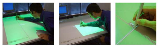
**Figure 4.5:** The user calibrates the image warping process by selecting targets projected by the (left) peripheral and (centre) foveal projectors. Each target (right) provides one point correspondence that is used in the homography calculation.
