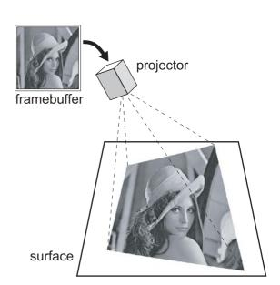
**Figure 4.1:** The rectangular image from a projector not aligned to the display surface will appear as a distorted quadrilateral.
