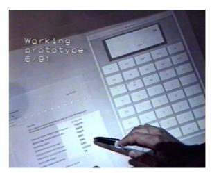
**Figure 2.15:** The DigitalDesk [Wel94]. Here the user has placed a paper document at a particular position on the desk at which a video camera is pointed. He can copy figures from the paper document to the calculator program on the right to save effort and avoid transcription errors.
