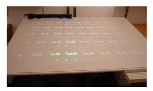
**Figure 5.6:** I tested the mapping from the digitizer and ultrasonic pens to the projector framebuffer using sets of correspondences between points in the framebuffer and points in pen co-ordinates. The points in pen co-ordinates were obtained by selecting regular a grid of points displayed from the projector.
