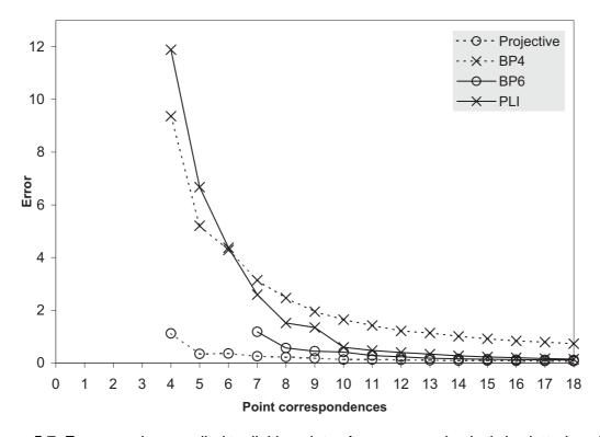
**Figure 5.7:** Four mappings applied to digitizer data. Average error in pixels is plotted against the number of point correspondences used to initialize the mapping. Projective, BP6 and PLI all converge to a low error. As expected, Projective produces the best results, achieving a low error level with only a few point correspondences.
