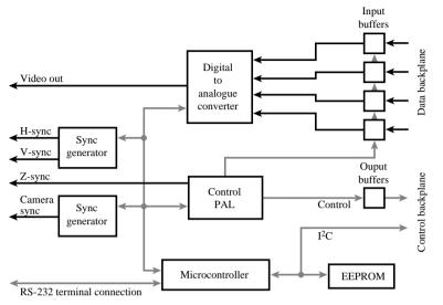
Figure 6: block diagram of the multiplexer board.
