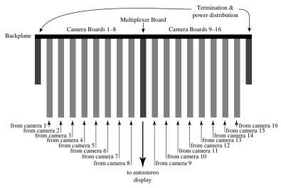
Figure 5: the maximum configuration of the autostereo camera system. Sixteen cameras' inputs are multiplexed into a single autostereoscopic video output. The backplane handles distribution of power, control and data. The two end circuit boards provide termination and power supply for the backplane.
