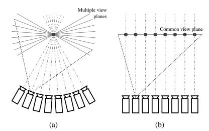
Figure 2: (a) shows the incorrect radial arrangement of cameras. This is incorrect because the multiple view planes from the different cameras are all displayed on a single screen plane, causing perspective distortion of the 3D picture. (b) shows the correct parallel arrangement of cameras. The common view plane is displayed on the single screen and the resulting 3D effect is good.
