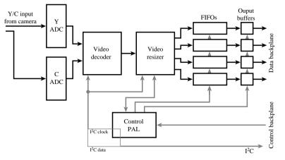
Figure 4: block diagram of the camera board.
