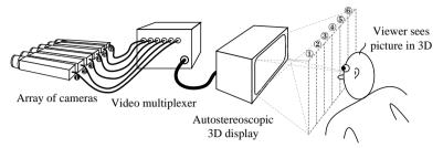
Figure 1: a six view autostereo display produces a different image on the screen for each of the six zones in space. Because his eyes are in different zones, the viewer sees one image with his left eye and a different image with his right eye, thus perceiving a 3D picture. The video multiplexer described in this report ensures that the image from each of the six cameras is visible in the appropriate zone.
