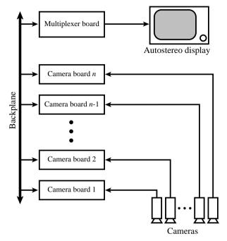
Figure 3: an overview of the autostereo camera system. Each of a set of cameras feeds a camera board. These are multiplexed together across a backplane, and the resulting output fed to the autostereo display.
