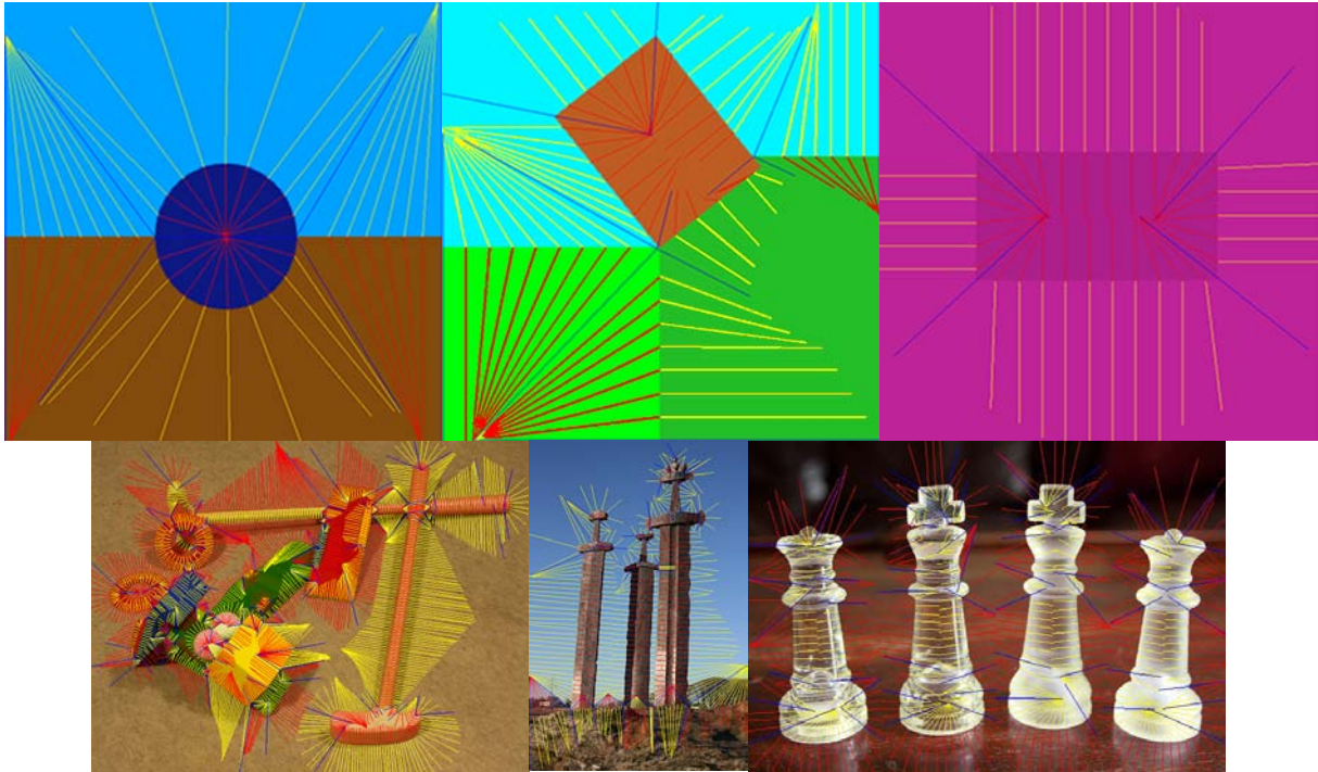
Figure 4.13: Rays shot from curve points extracted from images using the framework presented in Chapter 7. Rays related to corners and junctions, \hat{r}_i , are drawn with blue lines. The red and yellow lines relate to ‘normal’ rays r_i .
