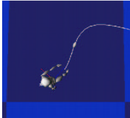
Figure 6.3: The next foot position is chosen at the start of each step. Here it is shown as the grey ellipsoid
