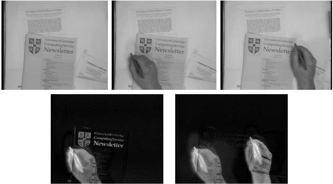
Figure 5. Inter-frame differencing. The frames in the second row show the differences between those above them in the first row.
