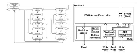
Fig. 1. (a) JTAG TAP state machine, (b) Simplified ProASIC3 security
