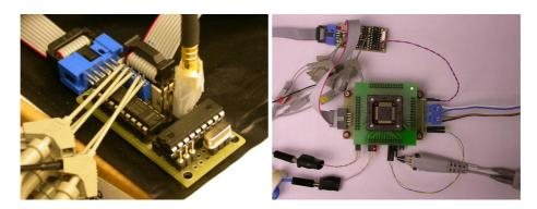
Fig. 2. Test setup: (a)control board, (b)DPA analysis
